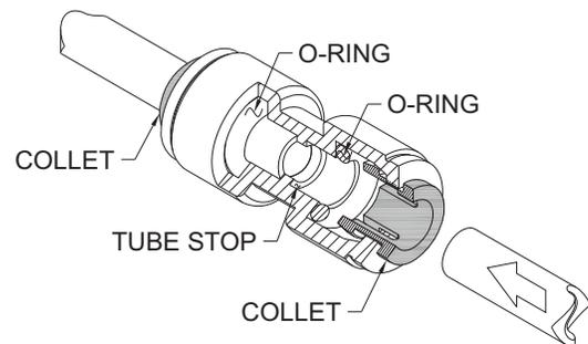
2. Pull on the fitted Tubing to ensure it is secure. Tube should not come free from the Fitting. Water test the connection assembly prior to leaving the site to ensure there are no leaks.
