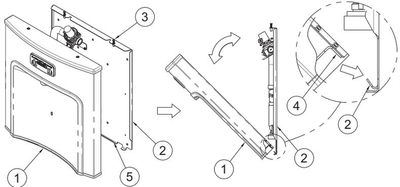
**13** Mount Water Cooler Access Panel to Water Cooler.
